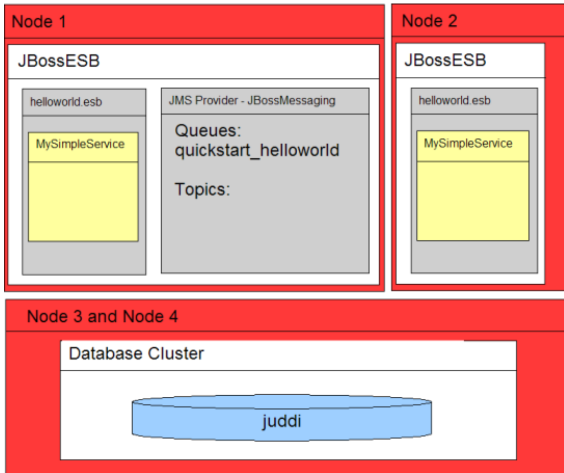
Figure 7.2. Two service instances each on a different node.
